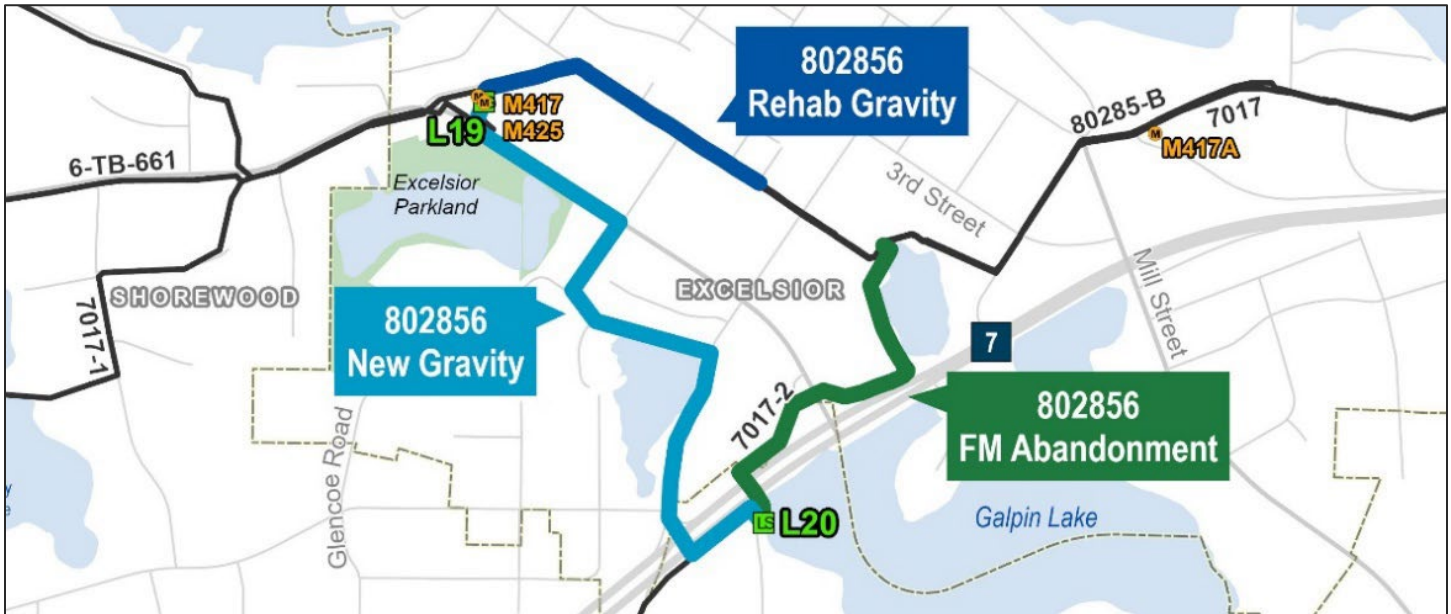
Map of Project #802856 in Excelsior showing new and rehabilitated gravity sewer and forcemain abandonment
