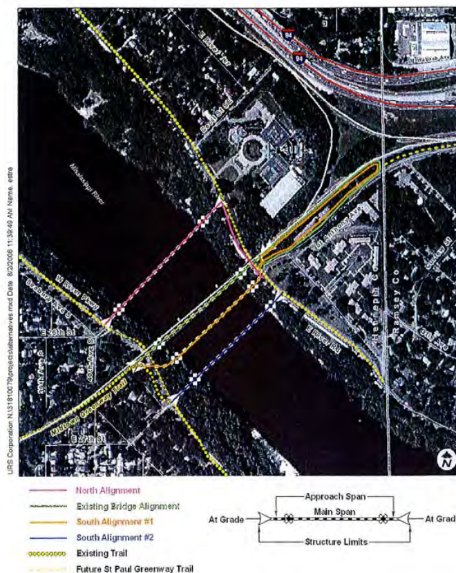
Figure 3: Bridge alternative alignments
