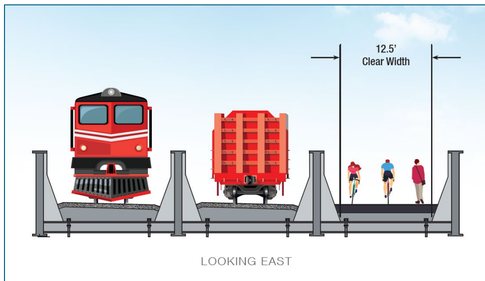
Figure 5: Conceptual section of girder bridge over I-94 of rail with trail concept
